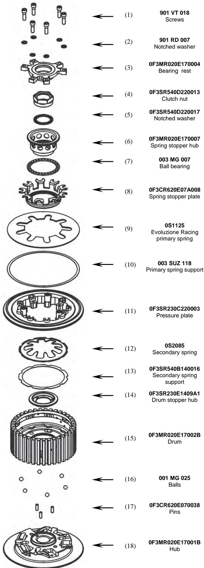
Pre-assemble the hub pack: place the 6 steel balls (16) at the bottom of the grooves of the hub (18) using a small amount of grease then fix the drum (15) onto the hub (18) with an M6x1 screw in an at-rest position.
