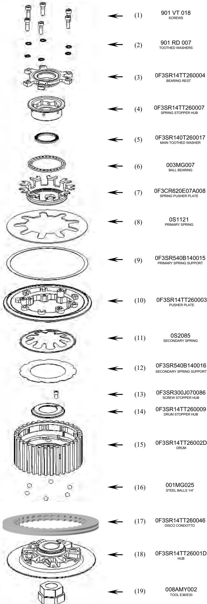
The Drum/Hub group is supplied pre-assembled. In case of need, as to check the ramps wear, please see hereinafter the specific procedure to disassemble the Drum/Hub group.
