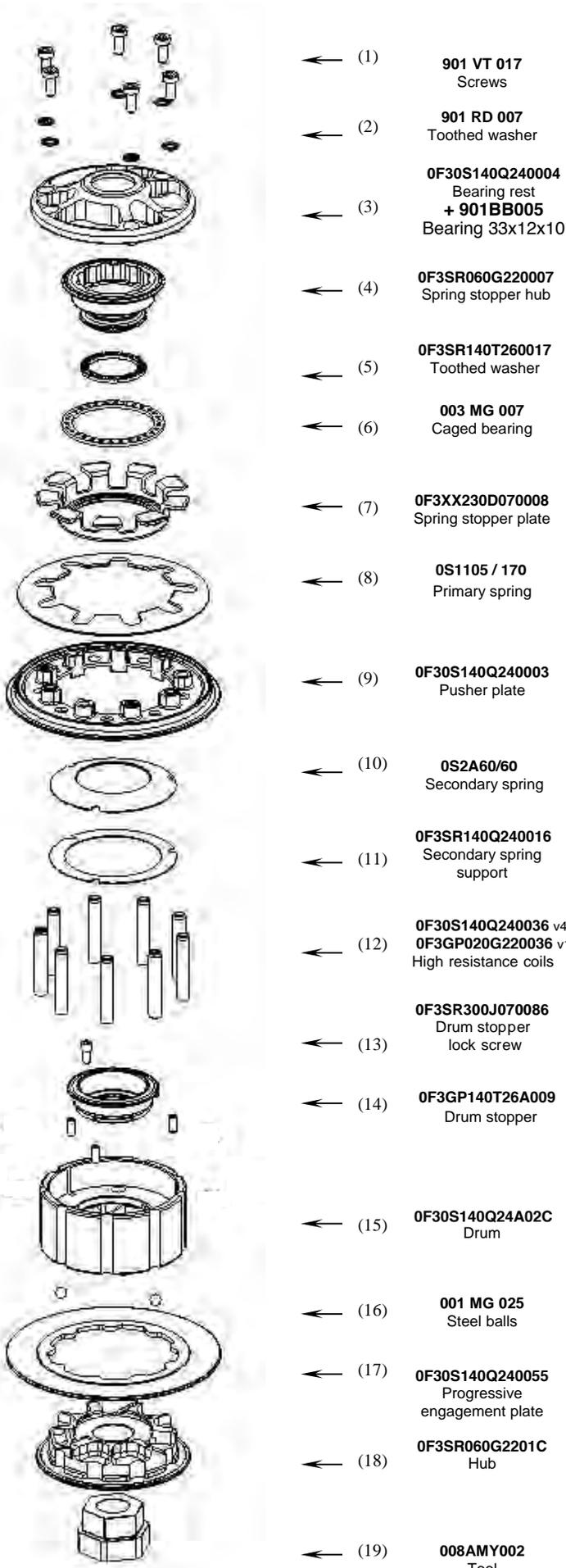
The Drum/Hub group (18/15) is supplied pre-assembled. **IN CASE OF NEED**, to perform a ramp condition inspection, see below the DRUM/HUB UN-INSTALL PROCEDURE.
